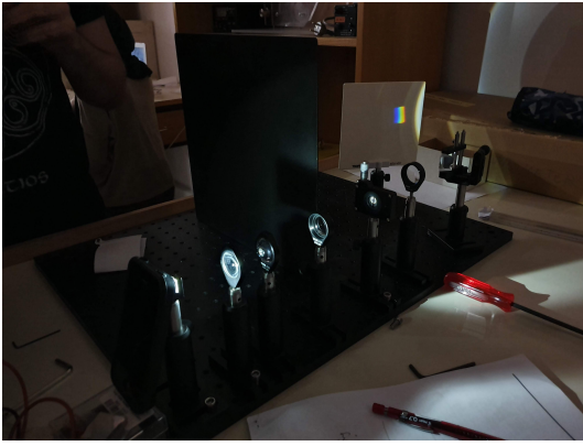
Figure 9. Separated Colors from Dispersion Prism
